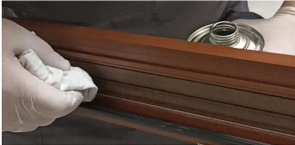
1. Clean the surface of the aluminum profile with isopropyl alcohol cleaner.
