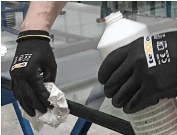
2. Clean the surface of the glass with isopropyl alcohol cleaner.
