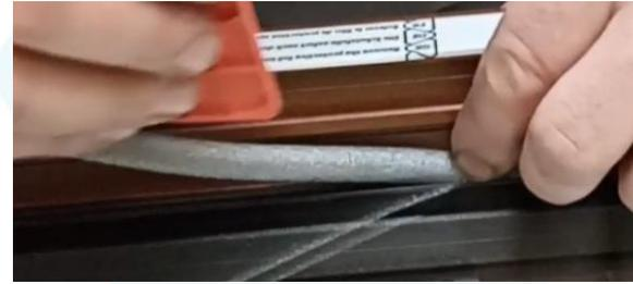
3. Put on foam seal between glass and aluminum profile on all profile circumference.
