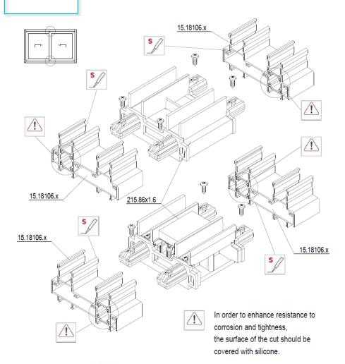
Screw the frame with the T-rex together. Use silicone for tight connections.
