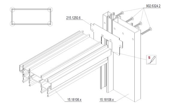
In order to connect corners, apply the glue on the surface of each corner connectors to seal the frame.
