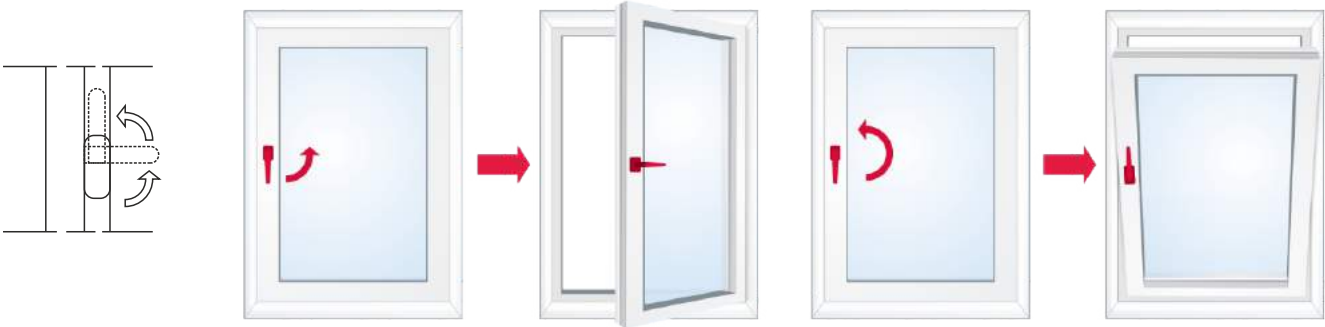
Turning - tilting window (closing - turning - tilting)
